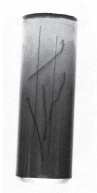
FIG. A1.25 NONRELEVANT INDICATIONS DUE TO CHANGE IN SECTION ON A SMALL PART (PRODUCED BY INDIRECT, CIRCULAR MAGNETIZATION, DC CONTINUOUS)
