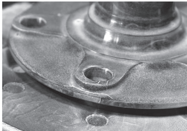
FIG. A1.4 CRANKSHAFT WITH VARIOUS LONGITUDINAL INDICATIONS
