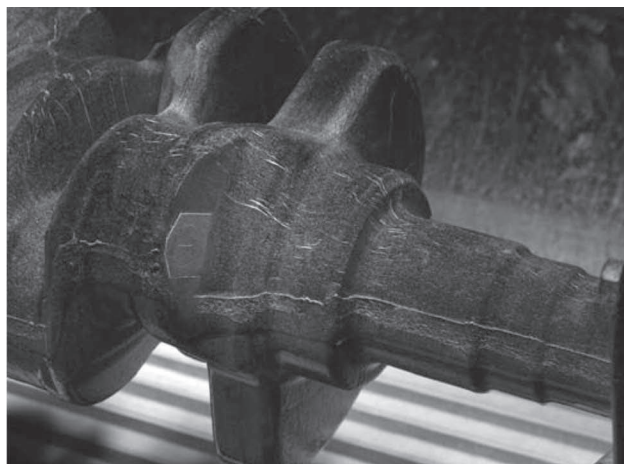
FIG. A1.4 CRANKSHAFT WITH VARIOUS LONGITUDINAL INDICATIONS
