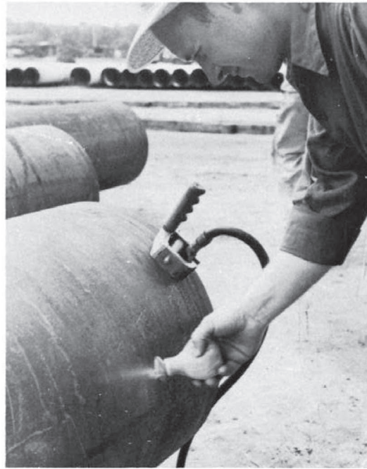
FIG. 5 DIRECT CONTACT MAGNETIZATION THROUGH MAGNETIC LEECH CLAMP OF PART
