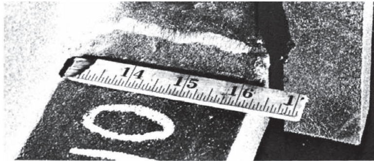
FIG. A1.19 INDICATION OF SURFACE CRACKS (PRODUCED BY CIRCULAR INDIRECT MAGNETIZATION, AC CONTINUOUS)
