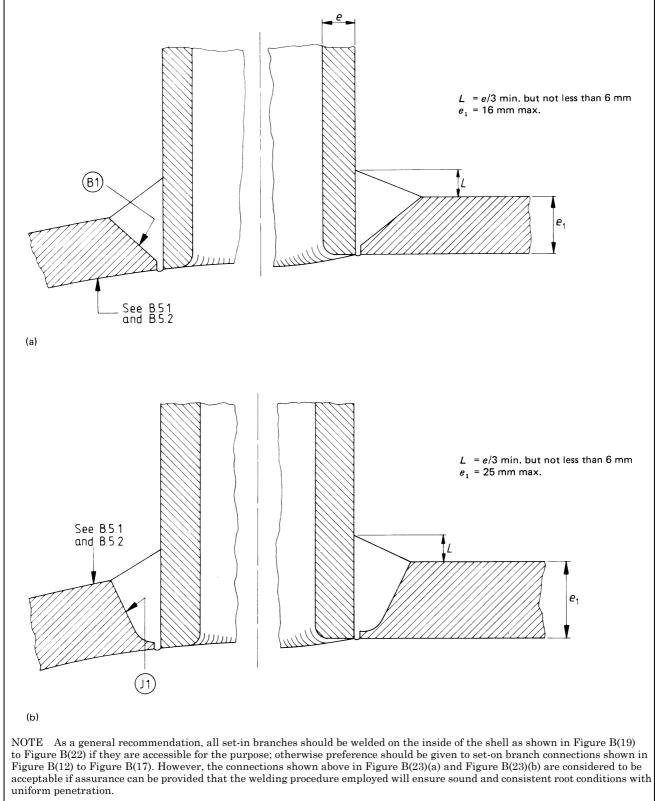
Figure B(23) — Set-in branches (full penetration welds, welded from one side only)
