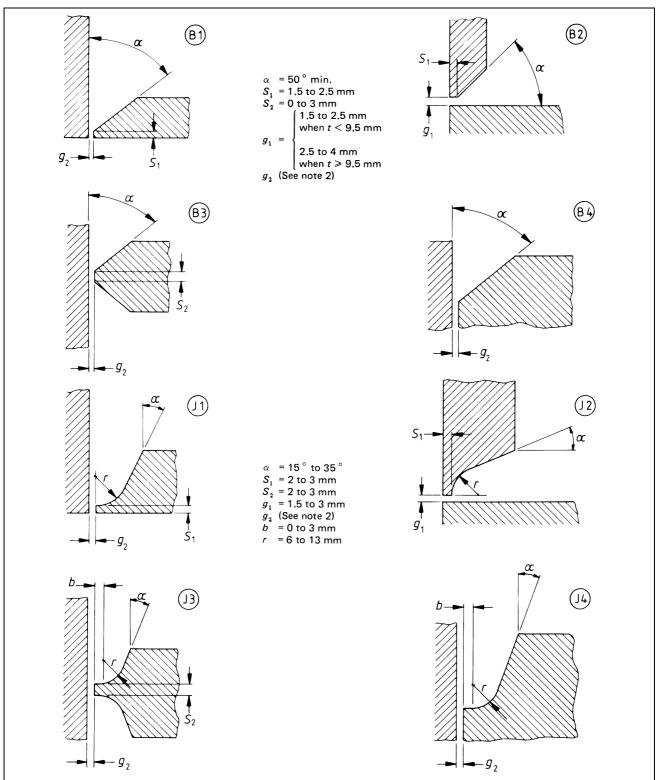
NOTE 1 These recommendations have been included for general guidance. Discretion should be used in applying the maximum and minimum dimensions quoted which are subject to variation according to the welding procedure employed (for example, size and type of electrodes), the position in which the welding is carried out and the practicability of carrying out satisfactory non-destructive testing, where necessary.
